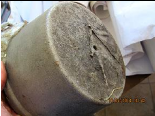
Bottom of pot with hole for detonator cord.
